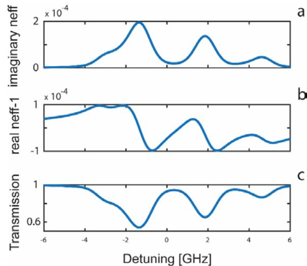
Fig. s1. (a-b) Simulated imaginary and real part of the refractive index of Rb<sup>85</sup>. (c) simulated transmission of our ACWG.
