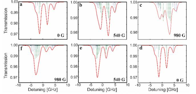
**Fig. s2.** Simulated transmission spectra of the ACWG with different magnetic fields (Red dotted lines), a-c right handed, d-f left handed polarization. The additional green lines represent the Rb85 transitions and the additional blue lines represent the Rb87 transitions.
