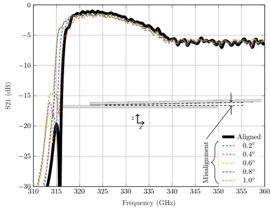
**Fig. S2.** Numerical simulations that investigate the impact of angular misalignment (i.e. rotation in the  $xz$ -plane) on the transmission efficiency of the vertical-coupling structure.
