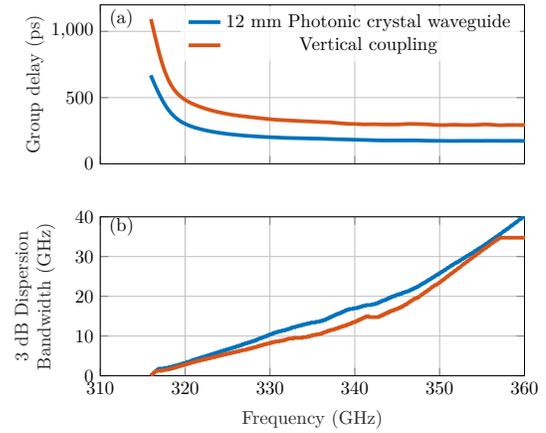
**Fig. S4.** An analysis of dispersion, showing (a) group delay, and (b) dispersion-limited 3 dB bandwidth, for a vertical coupling junction with  $L_{\text{overlap}} = 4$  mm, and  $d = 100$   $\mu\text{m}$ , as well as a single straight section of terahertz photonic crystal waveguide.
