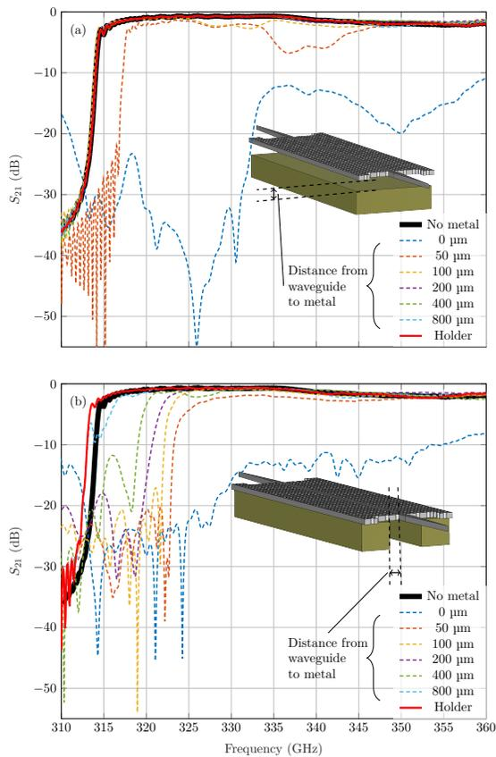
**Fig. S3.** Simulated interaction between terahertz photonic crystal waveguide and nearby metal, for (a) a metal block placed below the waveguide, in order to determine whether the sample holder's trench depth is sufficient, and (b) a bifurcated block of metal beneath, and in contact with the silicon, in order to determine whether the lateral separation between the waveguide and metal is sufficient. Both scenarios are illustrated as inset to the relevant plot.
