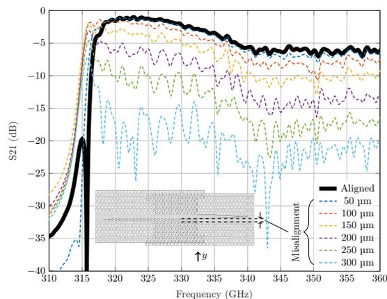
**Fig. S1.** The results of numerical simulations that probe the impact of horizontal misalignment. The physical situation under investigation is illustrated as inset.
