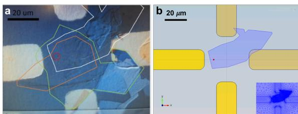
**Fig. S1.** a. Optical micrograph of the van der Waals heterostructure on the PMNT substrate. b. Simulated device in COMSOL (Inset: Mesh grids for the simulation on top view)
