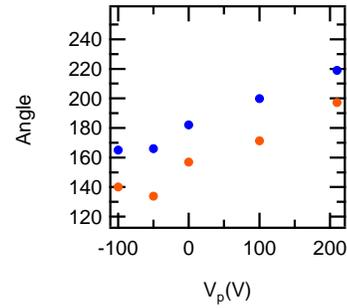
**Fig. S5.** Angle of emission of both the higher (blue) and lower energy peak (red) of the doublet as a function of applied voltage on the piezoelectric substrate.
