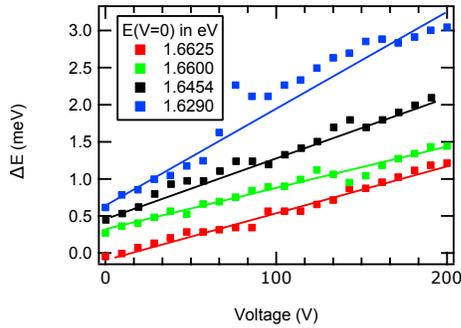
**Fig. S3.** Evolution of the emission energy shift as a function of strain for four different localized emitters exhibiting linear behavior. Solid lines are linear fit to the data. The emission energies of the different localized emitter are provided in the figure legend
