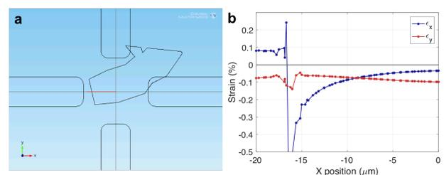
**Fig. S2.** a. Simulated device in COMSOL. b. Strain was calculated across the graphene flake as indicated by the red line in Fig.S2a
