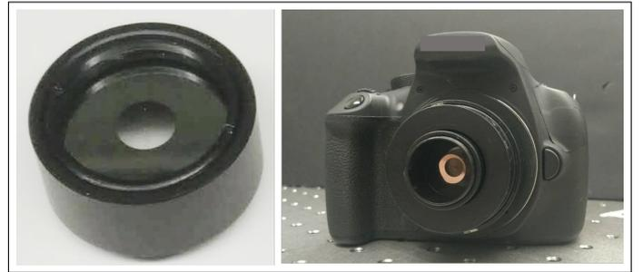
**Fig. S7.** Photographs of the prototype lens and the experimental setup using a DSLR camera body.
