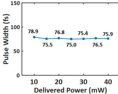
**Fig. S4. GRISM-delivered pulse width vs. delivered power.** The GRISM delivered consistent ~76fs pulses over the 10-40 mW power range.
