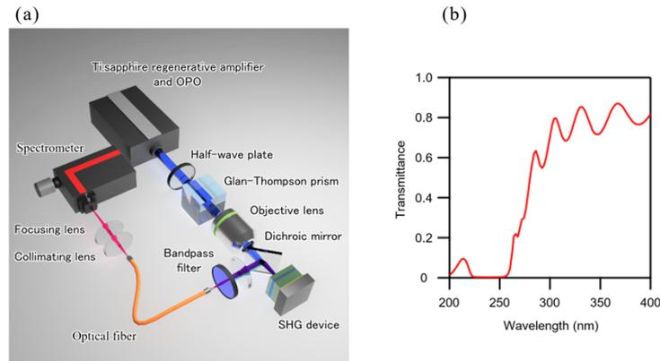
Fig. S1. Detail of optical experiment setup. (a) Schematic of optical experiment setup. (b) Transmission spectra. at  $45^\circ$  incidence of laboratory-made dichroic mirror.
