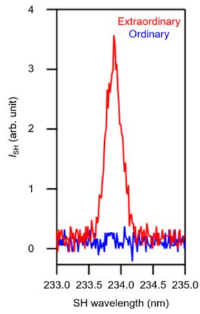
Fig. S2. Spectra of extraordinary and ordinary SH waves pumped by ordinary fundamental wave.
